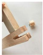
Figure 3-7 Horizontal Joint
